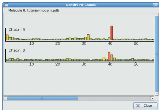
Figure 7 A typical validation graph. Bars represent individual residues in a chain, with an indication of quality for the residue being given by both the size and colour of the bar. The plot is interactive, i.e. clicking on a bar takes the user to the corresponding residue.
